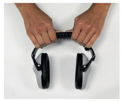
**Headband adjustment -** Apply a slight pressure against the curve of the headband and repeat the movement to the desired size. Wear it for a while to check effectiveness and comfort. If the headband is too tight, fold back the earmuffs and try again.
